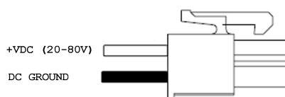
Figure 2.6: Power Connector used when controller is ordered without Galil Amplifiers
